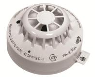
The XP95 I.S. Heat Detector operates by measuring heat levels with a single thermistor which gives a count output proportional to the external air temperature.
